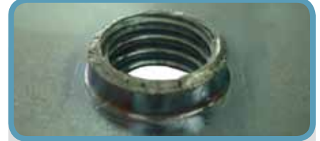
M8 x 1,25 thread • DC04 - Thickness: 2,5 mm • Thread depth: 6,5 mm Torque test: 20 N.m
