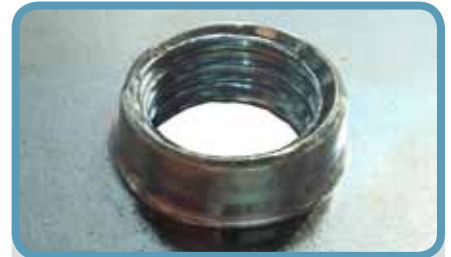
M10 x 1,50 thread • S420MC - Thickness: 3 mm • Thread depth: 6,5 mm Torque test: 75 N.m
